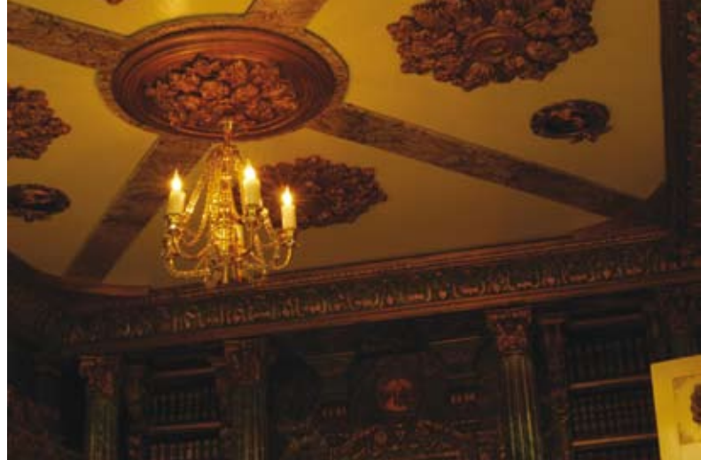
ABOVE LEFT: Tiny spotlights controlled by rheostats enhance the ceiling and coving details down to the sumptuously adorned pelmets over the window draw curtains. Most of the relief detail throughout the diorama was mastered by Bob and cast in resin. ABOVE RIGHT: The chandelier with candles hangs from the centre of the ornate ceiling. Again, the candles are controlled by rheostat.
